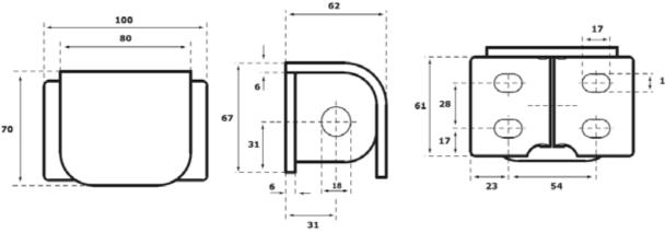
High security locking plates tested to EN12320 Grade 4. Manufactured from hardened steel with a durable zinc plate finish.
